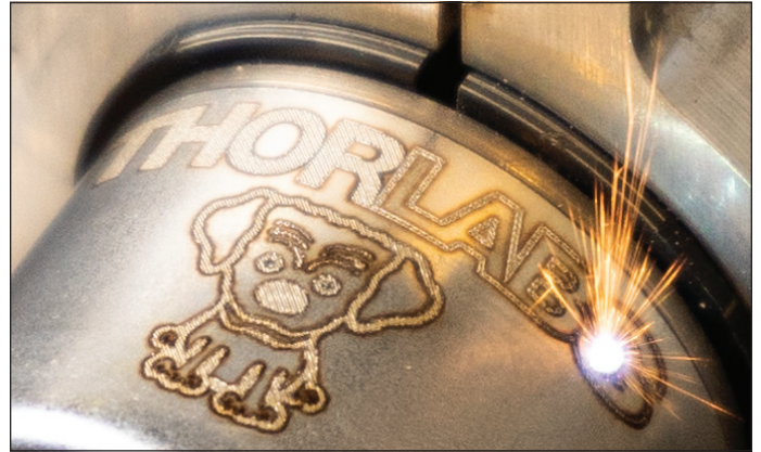
3-axis scanning systems use dynamic focusing to maintain a focused laser spot over a large, flat field or an arbitrary 3D surface.
