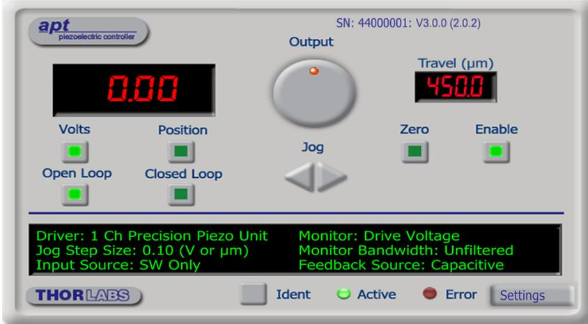
Fig. 3.5 GUI panel showing jog and ident buttons
