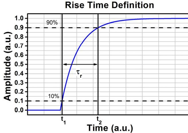
**Figure 9** The minimum rise time is the time required for the output signal to transition between points 10% and 90% up the rising edge of the curve generated in response to a step function input.
