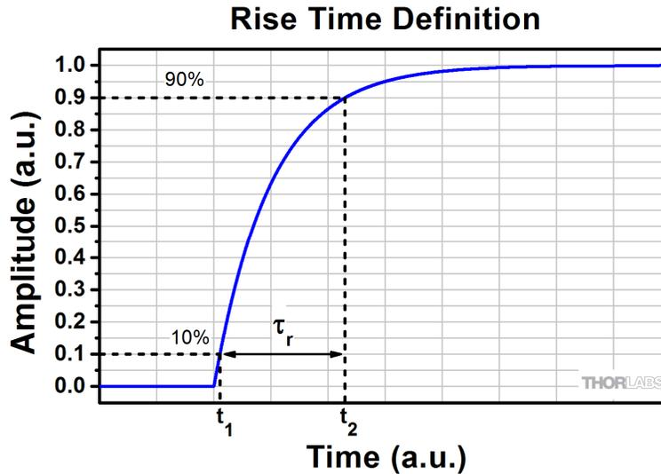
**Figure 1** Rise Time ( $\tau_r$ ) is defined as the time required for a signal to transition between points 10% and 90% up the rising edge of the curve.
