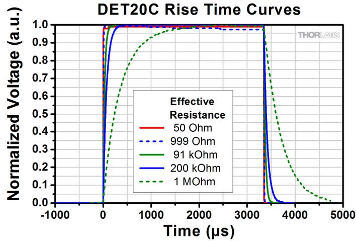
**Figure 13** Pulses output by a photodiode-based system were measured by an oscilloscope. The minimum rise times were measured between points 10% and 90% up the rising edges of the pulses, whose slopes varied with the effective load resistance.
