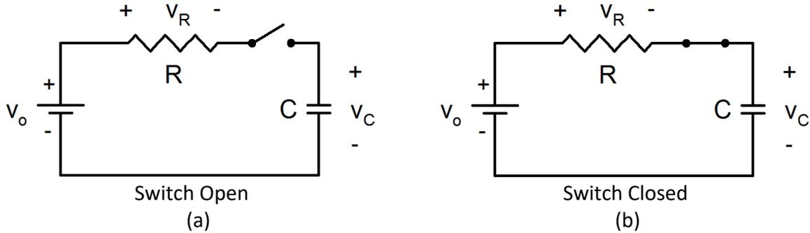
**Figure 7** An expression for rise time can be derived by considering the dynamic flow of charge in an RC low-pass filter circuit immediately after the open switch depicted in (a) is closed, as shown in (b).  $R$ ,  $C$ ,  $v_R$ , and  $v_C$  label the values of resistance, capacitance, and voltages. The voltage supplied by the source is  $v_o$ .
