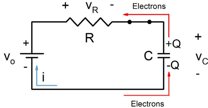
**Figure 8** After the switch closes, electrons flow to the bottom plate of the capacitor ( $C$ ) and away from the top plate. The accumulation of negative charge ( $-Q$ ) on the bottom plate and positive charge on the top plate ( $+Q$ ) causes a voltage to develop across the capacitor ( $v_C$ ). The labels  $R$ ,  $i$ ,  $v_R$ , and  $v_o$  indicate resistance, current<sup>7</sup>, voltage drops across the resistor, and the voltage supplied by the source, respectively.
