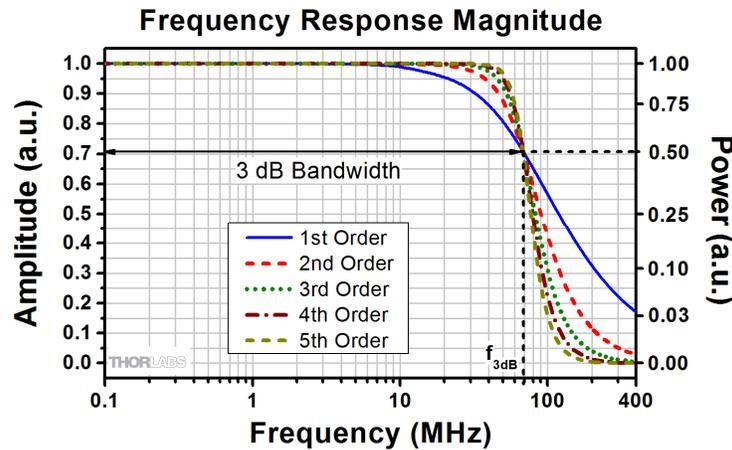
**Figure 5** The slope in the vicinity of the cutoff frequency ( $f_{3dB}$ ) can be used to classify the filter type. Filters with slopes of  $\omega^{-N}$  are  $N^{\text{th}}$  order low-pass filters. Note that all curves have a maximum value of one at DC and the same amplitude at  $f_{3dB}$ .
