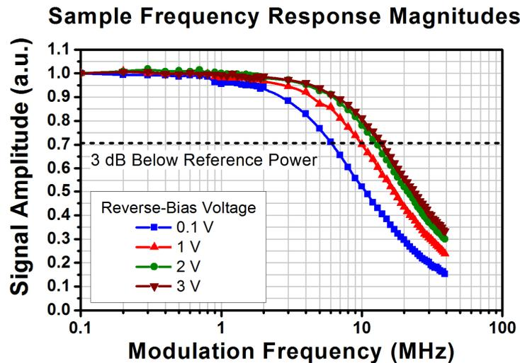
**Figure 15** Frequency response magnitude data were acquired using a photodiode-based system for cases in which four different reverse-bias voltages were applied across the photodiode. The 3 dB bandwidth was measured for each case. The lines connecting the data points are guides to the eye.
