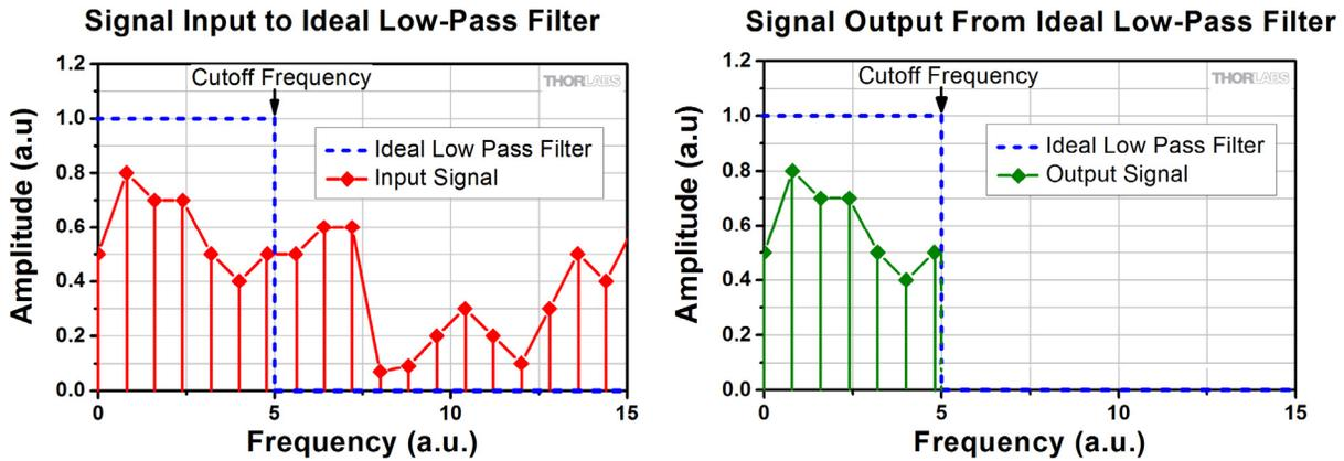
**Figure 4** When a signal input to an ideal low-pass filter contains components with frequencies above and below the cutoff frequency (left), the output signal will include only those components with frequencies less than or equal to the cutoff frequencies.
