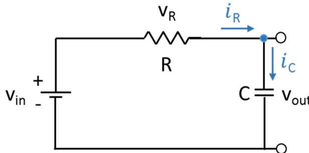
**Figure 12** The flow of current into and out of the node between the resistor and capacitor is noted for this RC low-pass filter circuit. Summing these currents is the first step in finding the frequency transfer function.
