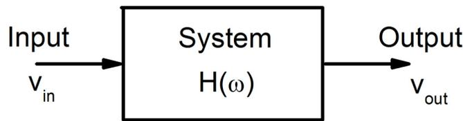
**Figure 11** A system provides the relationship between the input ( $v_{in}$ ) and output ( $v_{out}$ ) signals. A mathematical expression that relates any input signal with the resulting output signal is called a transfer function (H).
