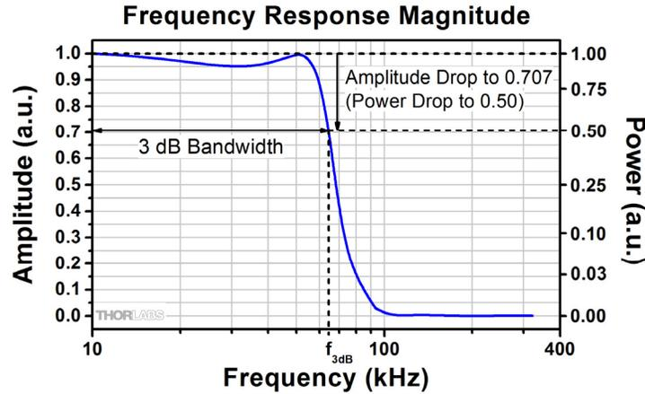
**Figure 6** Frequency magnitude response of the EF124 Low-Pass Electrical Filter showing a 3 dB cutoff frequency of approximately 68.4 kHz. Higher frequency components are strongly attenuated, while lower frequency components are preserved in the output signal. The cutoff frequency corresponds to a 0.707 multiplicative drop in voltage or current amplitude and a 0.5 multiplicative drop in power.
