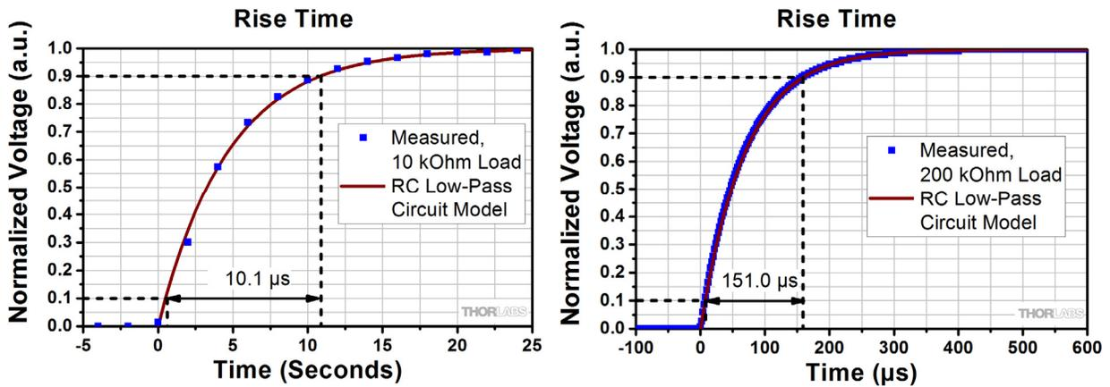
**Figure 14** Measurements of rise time, for two cases of effective load resistance, plotted with red curves calculated using the RC low-pass filter model (Eq. 22). The good fit of the curves to the data indicate the RC low-pass filter circuit is a good model for this system. Increasing the effective resistance increases the rise time. Shorter rise times may result in fewer data points measured along the rising edge.
