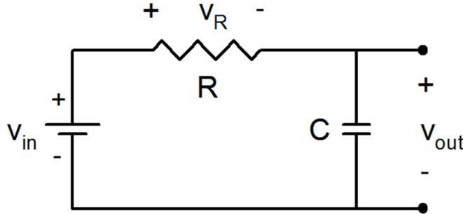
**Figure 10** An RC low-pass filter circuit can be seen as a system transferring an input, supplied by the source ( $v_{in}$ ), to an output ( $v_{out}$ ), measured across the capacitor (C). The resistor (R) is in series with the capacitor.
