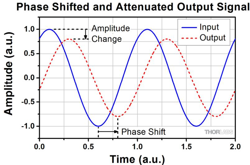
**Figure 2** Illustration of a signal output (red) by a system in response to the input (blue). In this example, points corresponding to particular radial values on the output signal occur at later times than the corresponding points on the input signal. The magnitude of the shift to later times is the phase delay. The system also attenuated the input signal, which reduced the comparative amplitude of the output signal.
