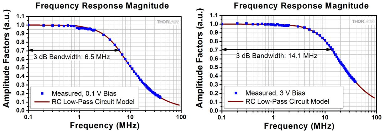
**Figure 16** Two frequency response magnitude data sets are shown, for cases of 0.1 and 3 V reverse-bias, with red curves calculated using the RC low-pass filter model (Eq. 46). The good fit of the curves to the data indicated the RC low-pass filter circuit is a good model for this system. Increasing the reverse bias increases the 3 dB bandwidth.
