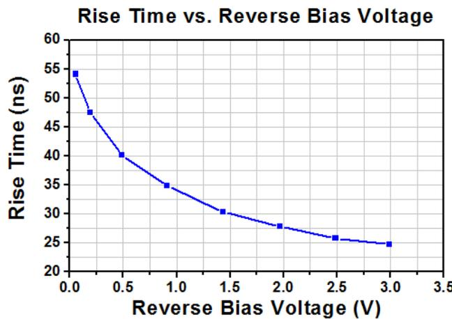
**Figure 17** Estimates of minimum rise time were calculated for each reverse bias voltage test case using the measured 3 dB bandwidth and Eq. 49.
