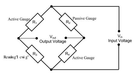
*Figure 4: Wheatstone bridge circuit with two active and two passive strain gauges*
