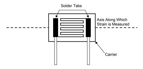
Figure 2: Schematic drawing of a metallic strain gauge
