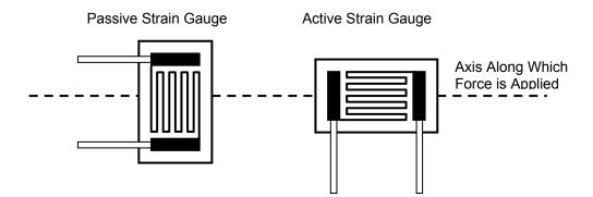
Figure 3: Passive strain gauge versus active strain gauge orientation
