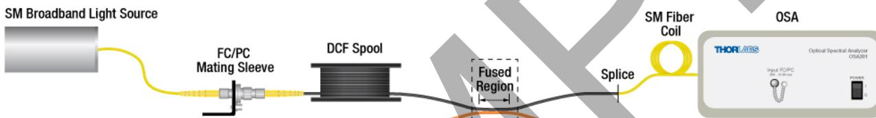
The single mode input of the coupler is connected to a Broadband Light Source (BBS) through an 405HP fiber and a spool of double-clad fiber (DCF). The single mode coupler output is spliced to a coiled 460HP patchcord (to insure cladding modes are stripped) that leads to an Optical Spectrum Analyzer (OSA). A spectrum is recorded before and after the coupler manufacturing process. The difference between the two spectra can be defined as either Insertion Loss (dB) or Transmission (%).
