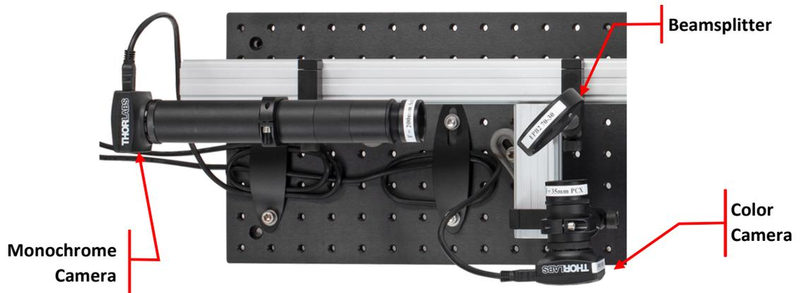
**Figure 1:** Color Camera and Beamsplitter Positioning
