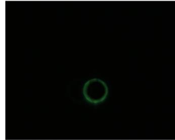
**Figure 7:** Top: Zero-Order Mask in SM1 Tube. Bottom Left: Image of Dot on BFP Camera; slightly out of focus because dot is  $\sim 2$  mm behind the exact BFP iris plane. Bottom Right: Image of Aperture Stop Closed Around Dot Showing Good Alignment; closing aperture stop slightly farther will result in darkfield imaging.
