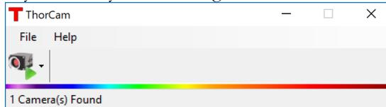
then click on the camera icon (on the left) and select a camera (with a number ending in “M” for Monochrome) from the drop-down menu.
