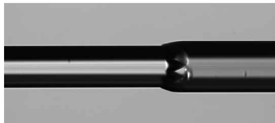
Image showing the stripped polyimide coating on a \varnothing 120 \mu\text{m} cladding and \varnothing 150 \mu\text{m} coating fiber. A clean, beveled edge (as shown here) is desirable for minimizing recoating defects after splicing.
